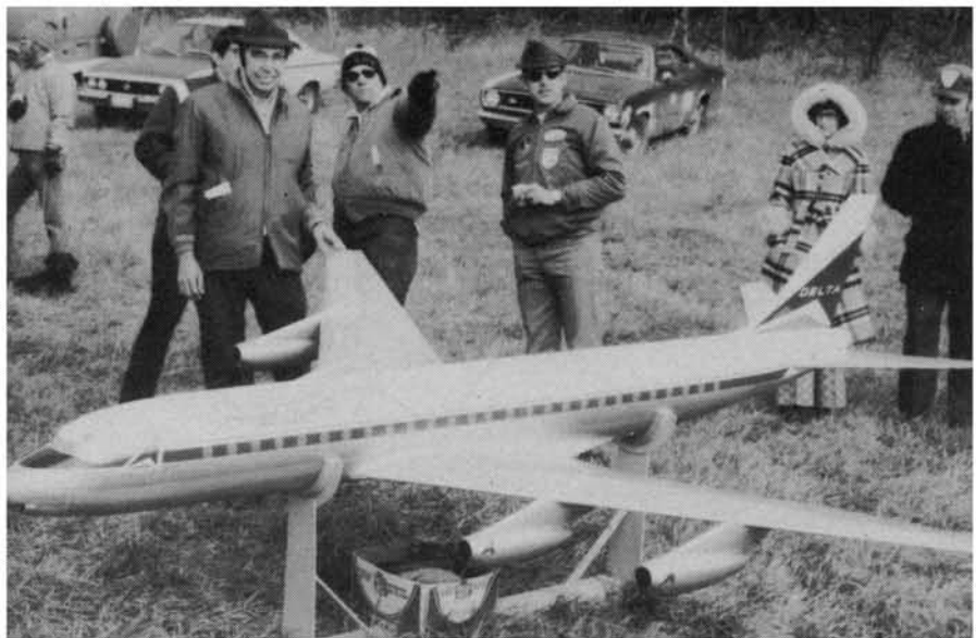
Displaying his wondrous creation is its designer. An engineer with NASA he employed a systems approach that took all aspects into consideration—the only way a complex project will reach happy fulfillment. The 10 1/2-pound, 10-ft. model has 14 sq. ft. of wing area—wing loading, 12 ounces.
